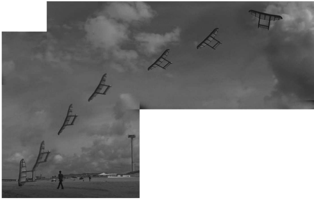
Fig. 12 Composite photo constructed from flight-test footage with v_W \approx 6 m/s, the flight time captured in this figure is approximately 12 s.
